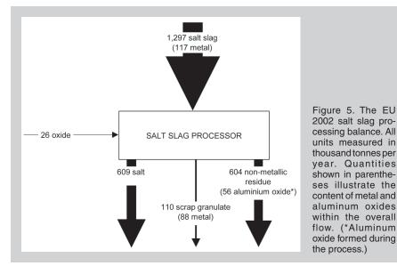
of the metal inventory is completely converted into oxide, although most of the oxidized metal ends up in slightly differing chemical compositions. The whole non-metallic residue is filtered and washed to a final salt content of 0.2%, reflecting target values of the cement industry that apply to this oxide blend product. A salt balance is used to determine the amount of additional salt needed by refiners and remelters.
