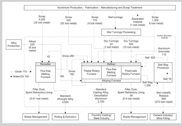
Figure 6. The material flows into, out of, and within the EU aluminum recycling industry. All units measured in thousand tonnes per year. Values in parentheses represent the amount of metallic aluminum lost due to oxidation. Spent refractory lining does not include any furnace material.
