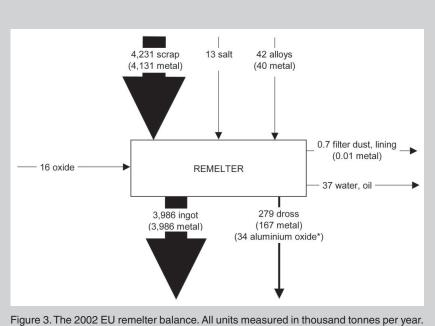
Figure 3. The 2002 EU remelter balance. All units measured in thousand tonnes per year. Quantities shown in parentheses illustrate the content of metal and aluminum oxides within the overall flow. (\*Aluminum oxide formed during the process.)
