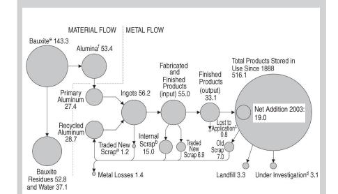
Figure 1. Global aluminum flow.<sup>1</sup> All units measured in million tonnes per year. Values might not add up due to rounding. a–Aluminum in dross; b–not taken into account in statistics; c–such as powder, paste, and deoxidation aluminum (metal property is lost); d–area of current research to identify final aluminum destination (reuse, recycling, or landfilling); e–includes, depending on the ore, between 30% and 50% alumina; f–includes, on a global average, 52% aluminum.
