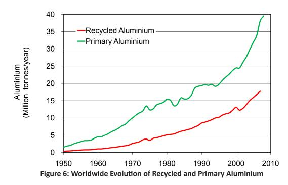
The aluminium recycling industry has almost quadrupled its output from 5 million tonnes in 1980 to close to 18 million tonnes in 2007 from old and
